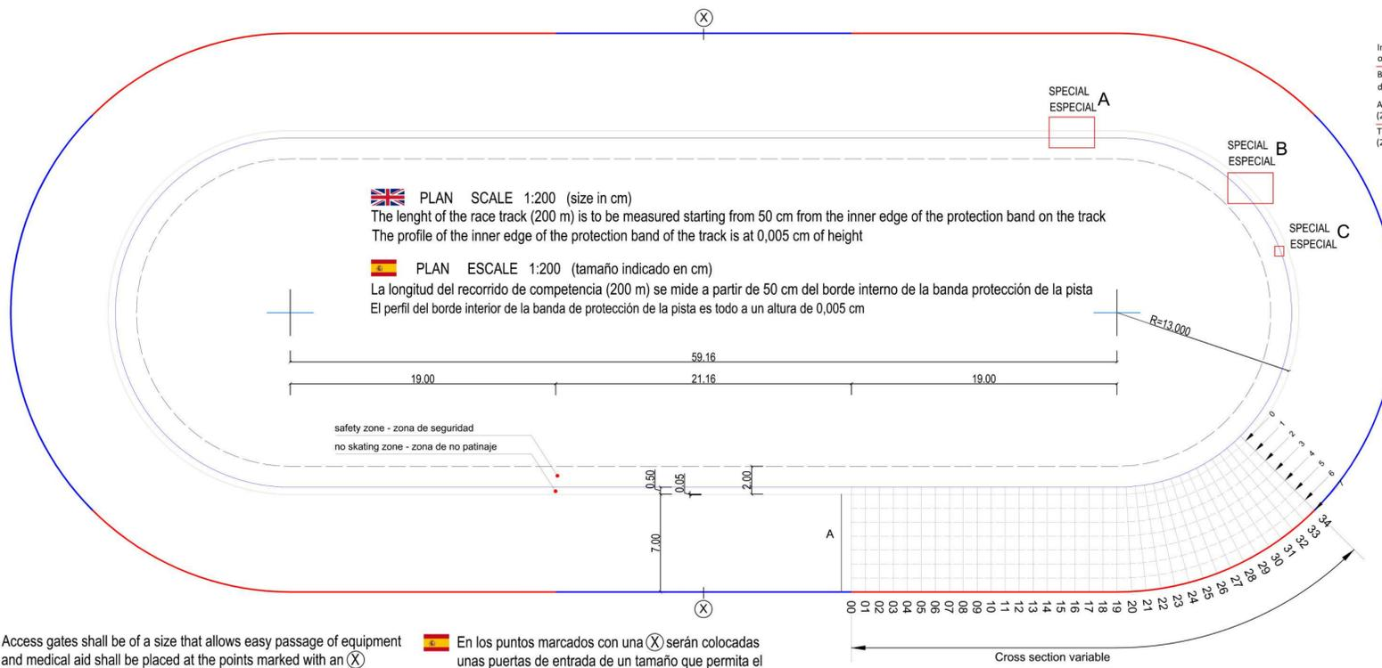
Access gates shall be of a size that allows easy passage of equipment and medical aid shall be placed at the points marked with an (X)
